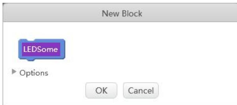
This instruction should have one digital parameter. After adding the name of the LEDSome, click "Options", then click the "Add a digital state" as shown in the rounded edge icon.
