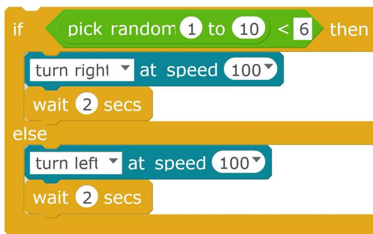
The robot will pick a number from 1 to 10. If the number is less than 6 (i.e. 1, 2, 3, 4, 5), the robot will turn right. On the contrary, if the number is not less than 6 (i.e. 6, 7, 8, 9, 10), the robot will turn left. The program is as below:
