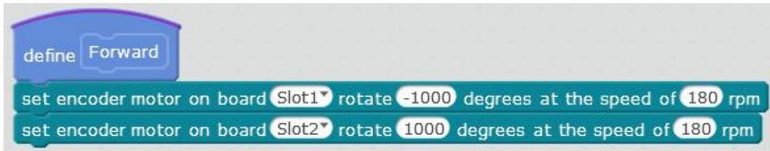
The speed has been set at 180, so when we use the Forward command, Ranger can only go forward at the fixed speed of 180. If you want to change the speed, you may need to use another new block.
