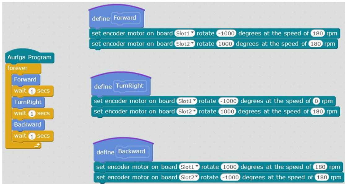
When we want to make Ranger carry out more complex movements, with [Make a Block] command, the program now becomes simpler and tidy, making it very easy to read.
