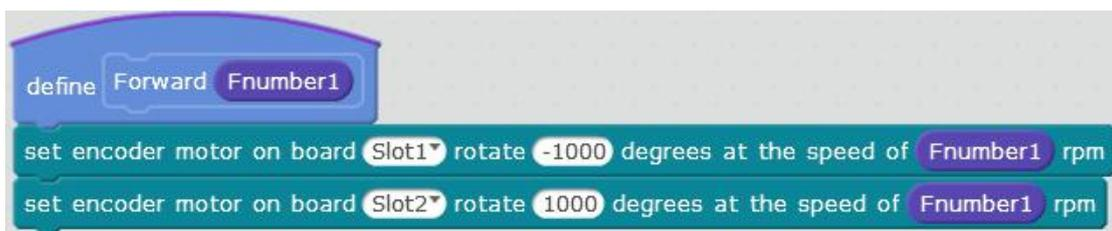
8. Upon completion of the change, the Forward command has the function to input parameters, such as Forward 100, meaning Fnumber1 value is 100, and while using [Fnumber1], the value of the parameters will be replaced by 100. Simply put, the Ranger's two encoder motors will rotate at a speed of 100. With parameters, the blocks will have more changes.
