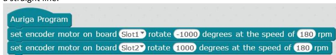
What about retreating in a straight line? Having Slot1 set at 1000 degrees and Slot2 set at -1000 degrees, the program is shown in the diagram below:
